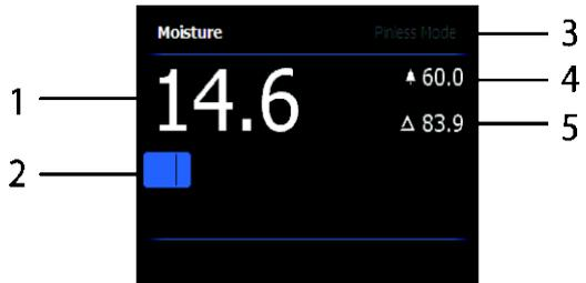
**Fig. 5-1(b) Moisture-only Mode**
