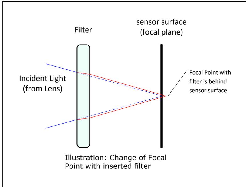
In this example when a glass filter is inserted between the lens and the camera sensor, the focal point is now about 1/3 of the filter thickness behind the sensor plane.
