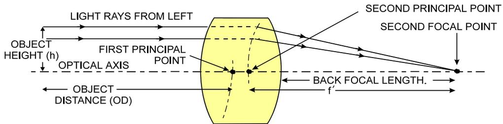
Figure 1: Primary Points in a Lens System
